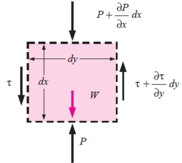
Forces acting on a differential control volume in the natural convection boundary layer over a vertical flat plate
