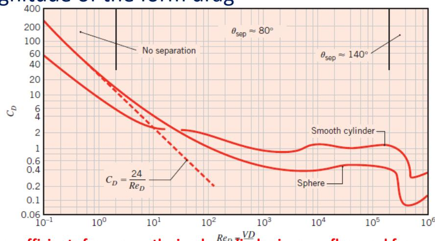
**Drag coefficients for a smooth circular cylinder in cross flow and for a sphere.**
