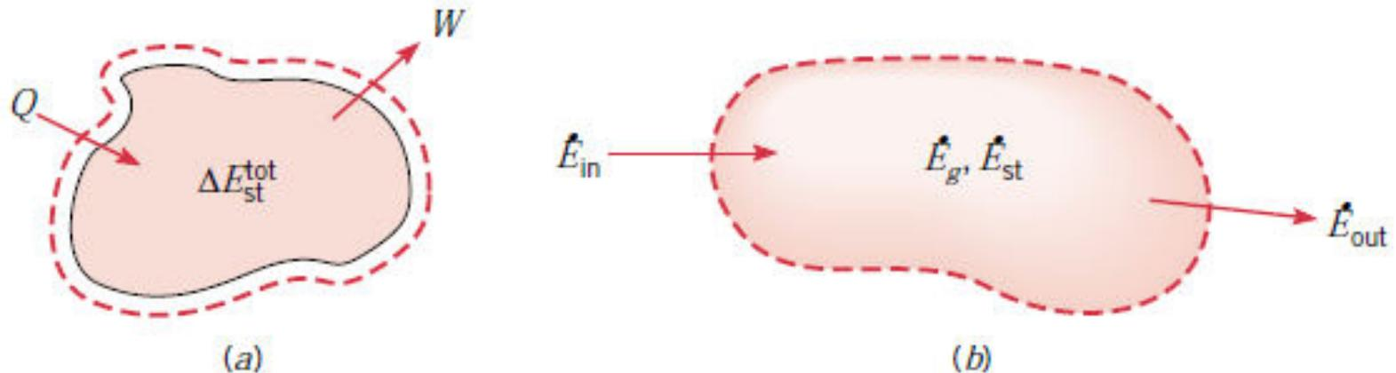
*Conservation of energy for a) closed system over a time interval b) for control volume at an instant*
