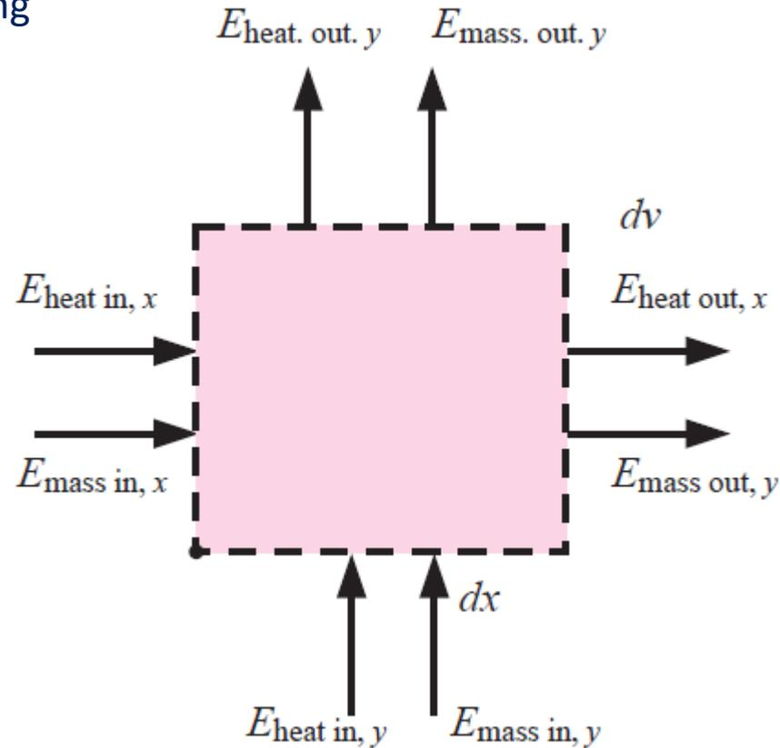
$$(\dot{E}_{\text{in}} - \dot{E}_{\text{out}})_{\text{by heat}} + (\dot{E}_{\text{in}} - \dot{E}_{\text{out}})_{\text{by work}} + (\dot{E}_{\text{in}} - \dot{E}_{\text{out}})_{\text{by mass}} = 0$$
