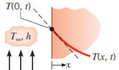
Boundary condition of third kind corresponds to existence of convective heating or cooling of surface and is obtained from surface energy balance
