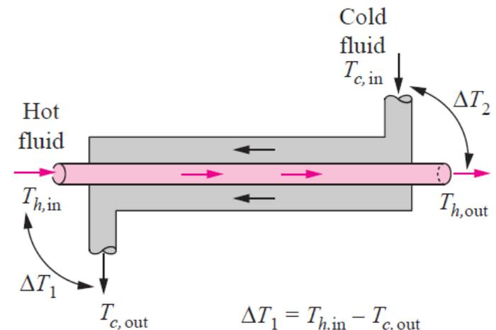
$$\Delta T_1 = T_{h,in} - T_{c,out}$$
