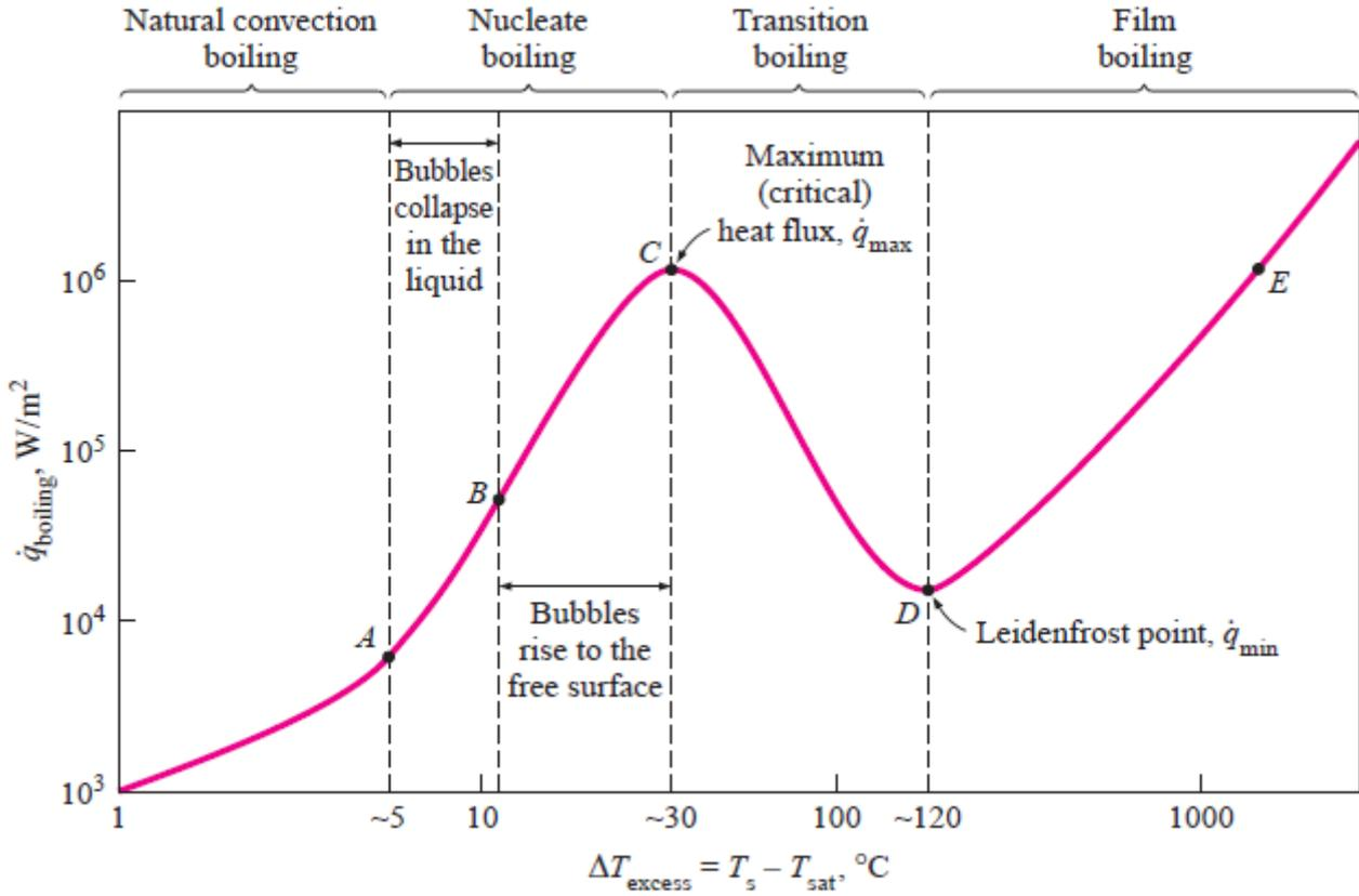
Typical boiling curve of water at 1 atm pressure
