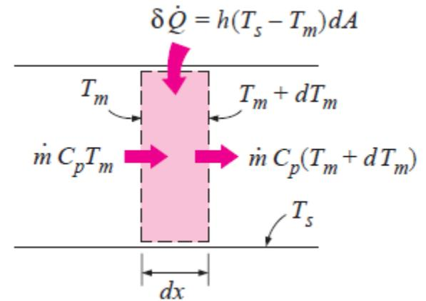
$$\frac{\partial T}{\partial x} = \frac{dT_s}{dx} = \frac{dT_m}{dx} = \frac{\dot{q}_s p}{\dot{m} C_p} = \text{constant}$$
