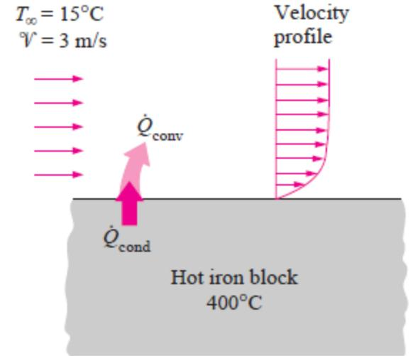
The cooling of a hot block by forced convection
