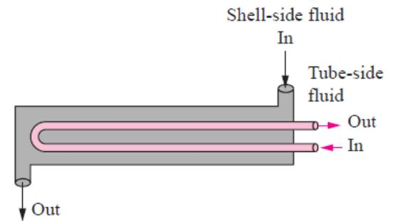
(a) One-shell pass and two-tube passes
