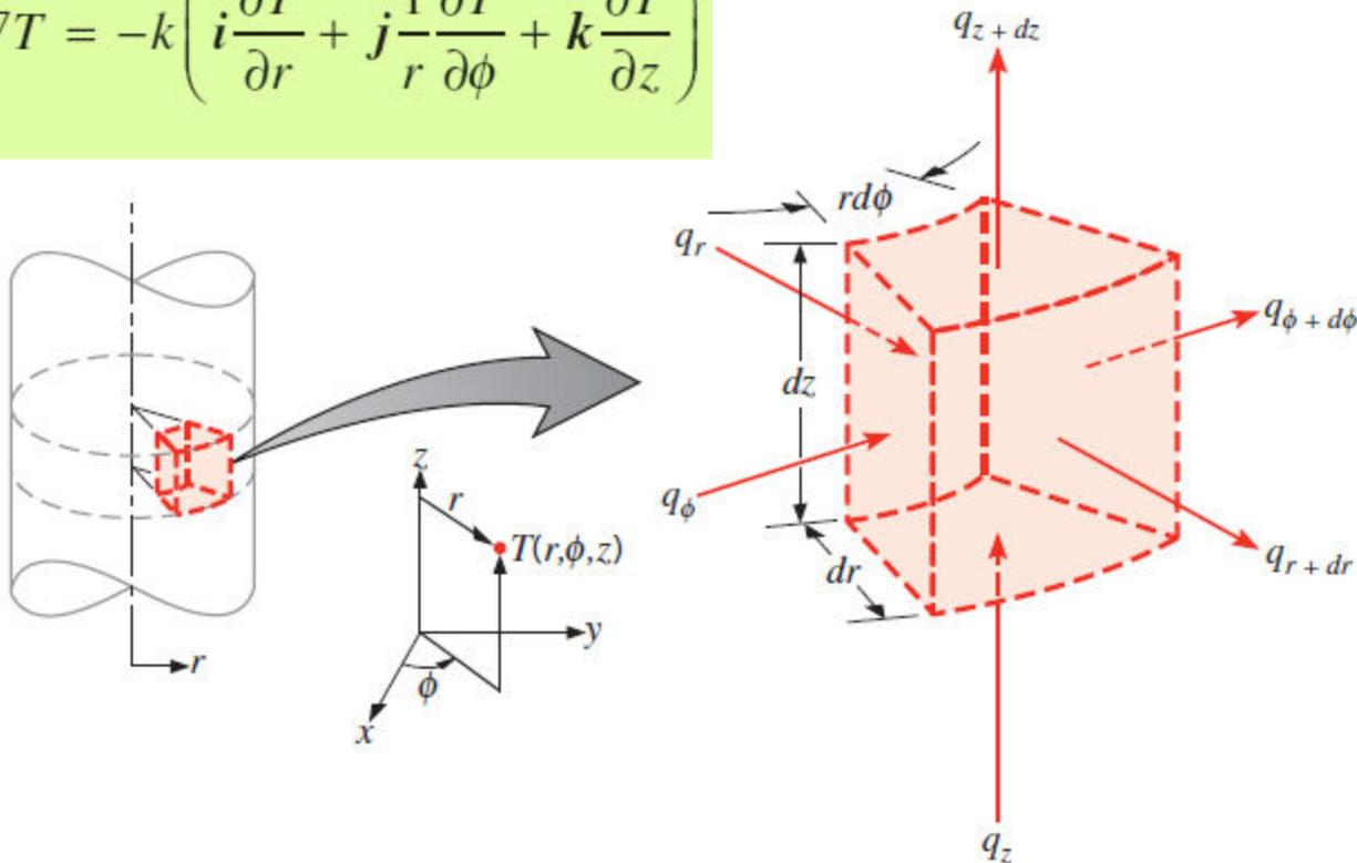
Differential control volume  $dr, rd\phi, dz$  for conduction analysis in cylindrical coordinates
