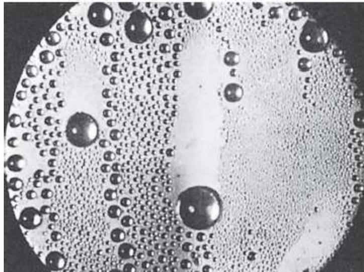
Dropwise condensation of steam on a vertical surface
