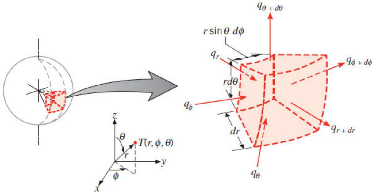
Differential control volume  $dr. r \sin \theta d\phi. r d\theta$  for conduction analysis in spherical coordinates
