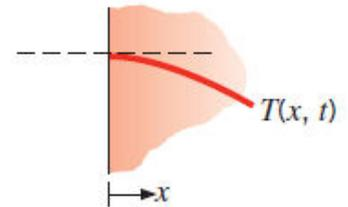
A special case of second condition exists for perfectly insulated or adiabatic surface
