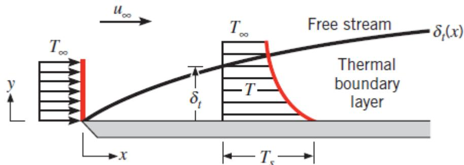
Thermal boundary layer development on an isothermal flat plate
