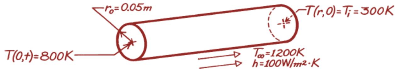
$$\rho = 7832\text{ kg/m}^3, k = 51.2\text{ W/m}\cdot\text{K}, c = 541\text{ J/Kg}\cdot\text{K}, \alpha = 1.21 \times 10^5\text{ m}^2/\text{s}$$
