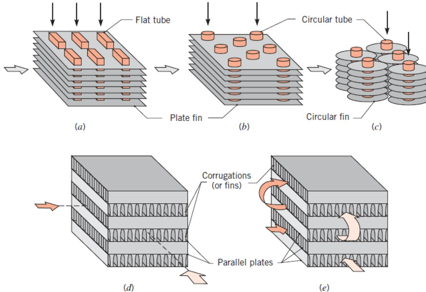
Compact heat exchanger cores. (a) Fin-tube (flat tubes, continuous plate fins). (b) Fin-tube (circular tubes, continuous plate fins). (c) Fin-tube (circular tubes, circular fins). (d) Plate-fin (single pass). (e) Plate-fin (multipass)
