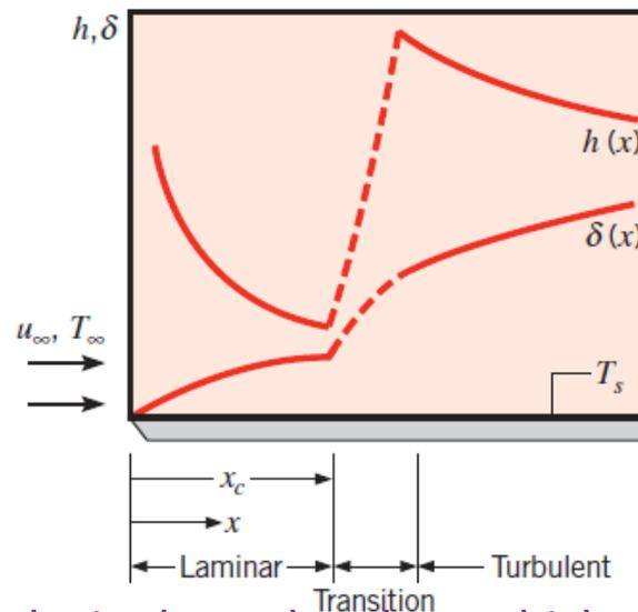
Variation of velocity boundary layer thickness  $\delta$  and the local heat transfer coefficient  $h$  for flow over an isothermal flat plate
