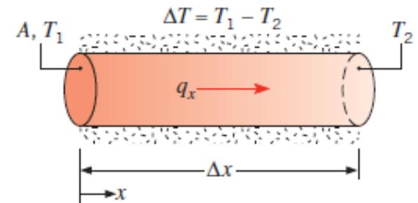
*We are able to measure the heat transfer rate  $q_x$ , and seek to determine how  $q_x$  depends on the following variables:  $\Delta T$ , the temperature difference;  $\Delta x$ , the rod length; and  $A$ , the cross-sectional area*
