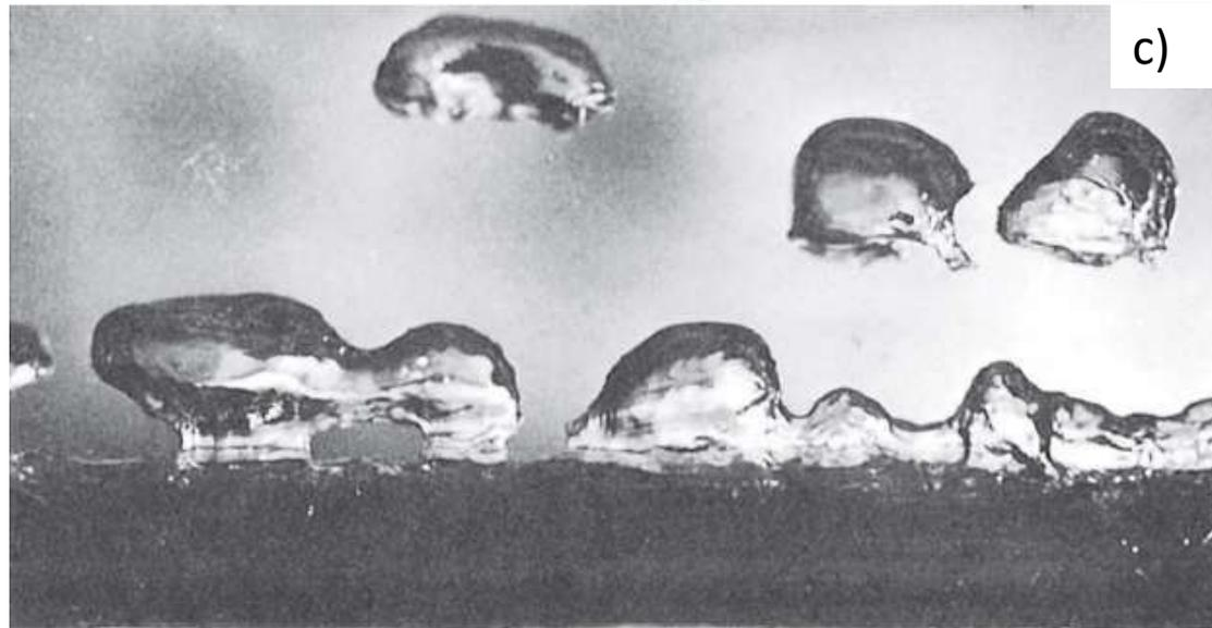
**(a) nucleate boiling, (b) transition boiling, and (c) film boiling**
