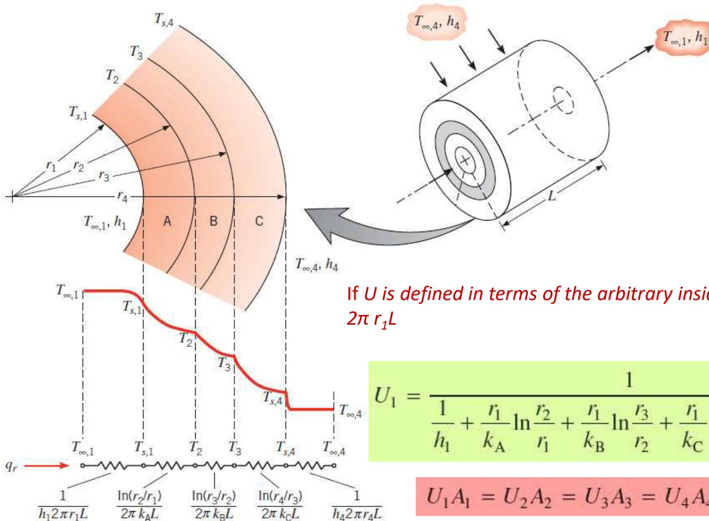
$$U_1 = \frac{1}{\frac{1}{h_1} + \frac{r_1}{k_A} \ln \frac{r_2}{r_1} + \frac{r_1}{k_B} \ln \frac{r_3}{r_2} + \frac{r_1}{k_C} \ln \frac{r_4}{r_3} + \frac{r_1}{r_4} \frac{1}{h_4}}$$
