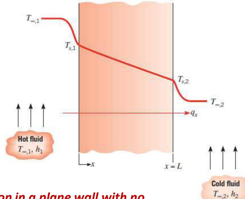
**for one-dimensional, steady-state conduction in a plane wall with no heat generation, the heat flux is a constant, independent of x**
