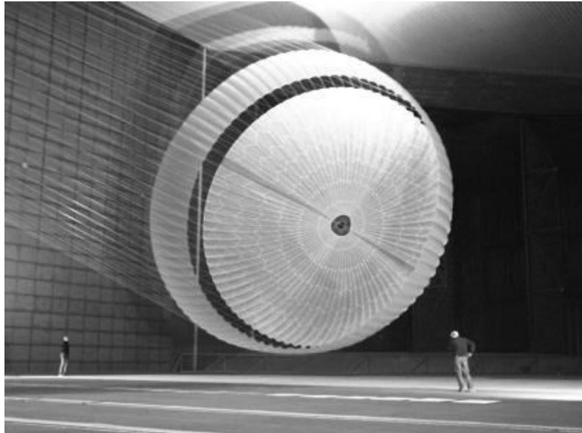
*Large parachute being tested at NASA facility for MARS mission*
