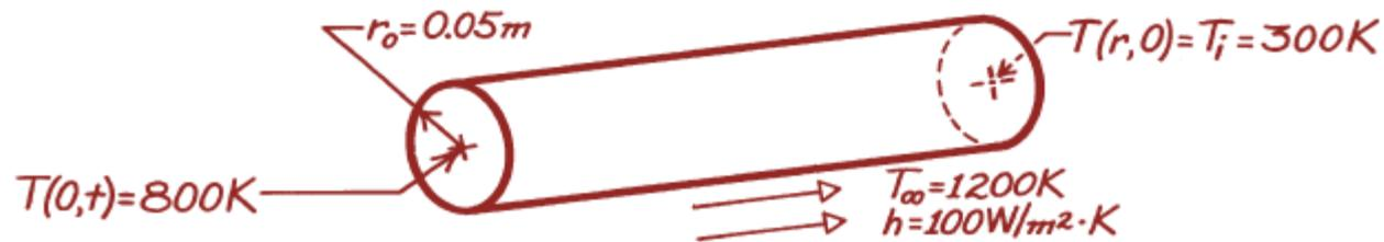
$$\rho = 7832 \text{ kg / m}^3, k = 51.2 \text{ W/m.K}, c = 541 \text{ J/Kg K}, \alpha = 1.21 \times 10^5 \text{ m}^2/\text{s}$$
