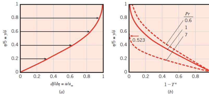
Similarity solution for laminar flow over an isothermal plate. (a) The  $x$ - component of the velocity. (b) Temperature distributions for  $Pr = 0.6, 1, \text{ and } 7$
