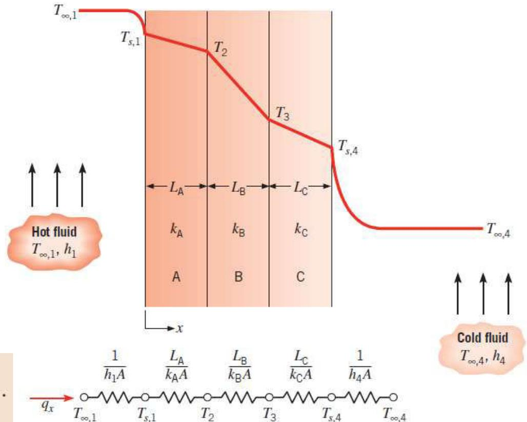
$$q_x = \frac{T_{\infty,1} - T_{\infty,4}}{[(1/h_1A) + (L_A/k_A A) + (L_B/k_B A) + (L_C/k_C A) + (1/h_4A)]}$$
