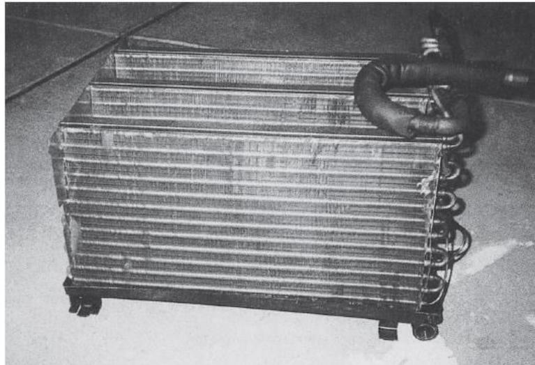
A gas-to-liquid compact heat exchanger for a residential air-conditioning system
